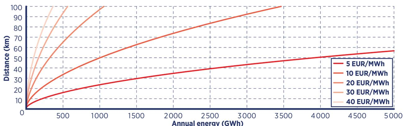
**Note:** The cost of transmission includes the construction cost and the cost of pumping. Construction costs for district heating pipes have been taken from Svensk Fjärrvärme AB (2007), updated following Sánchez-García (2017) and amortised at 30 years with an interest rate of 5%. Pumping cost have been calculated assuming an electricity price of USD 11/MWh. Furthermore, it has been assumed that the energy transported through the pipeline varies sinusoidally through the year (Phetteplace, 1995).
