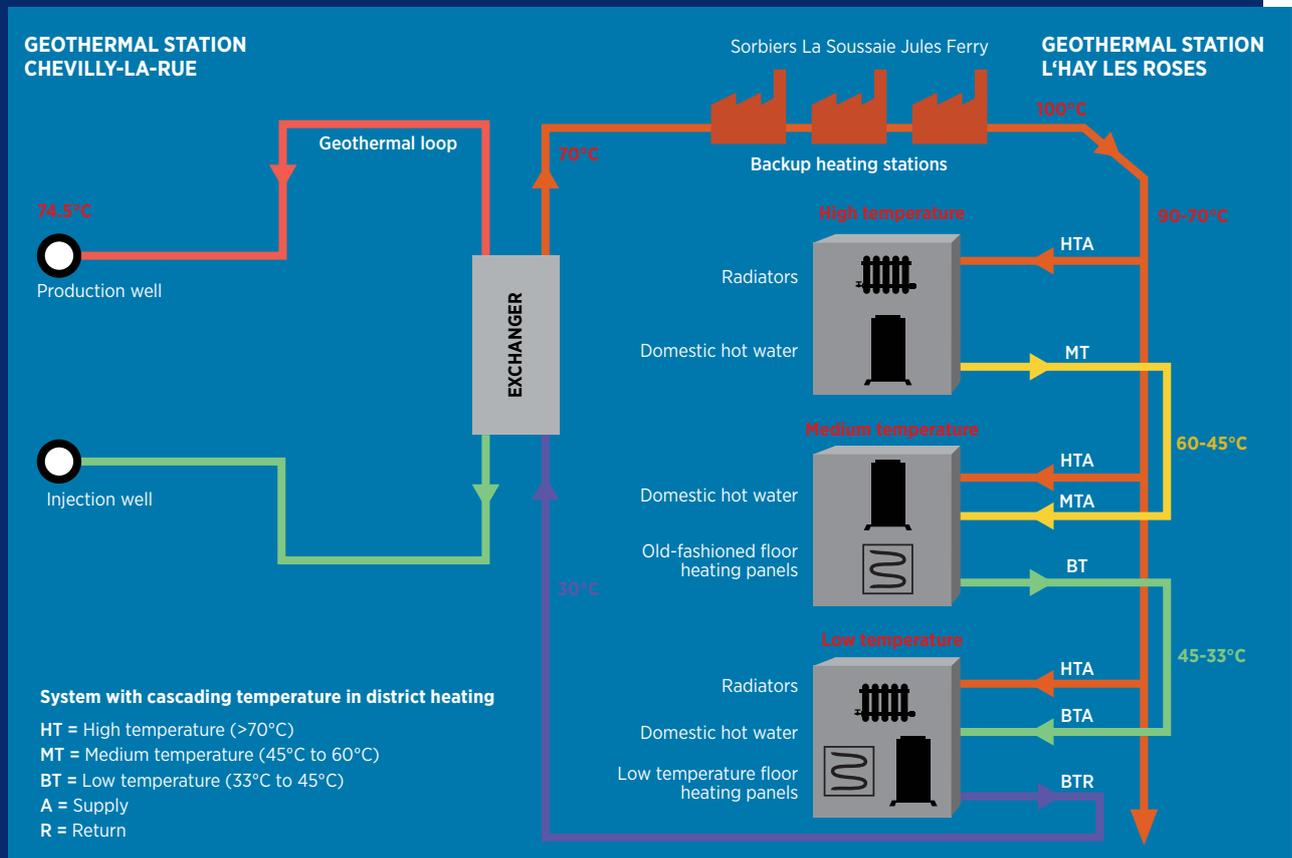
The Île-de-France subsurface is rich in geothermal energy. The utility SEMHACH operates in the Paris suburban municipalities of Chevilly-Larue, L'Haÿ-les-Roses and Villejuif and implements a cascading multi-temperature district heating system, where five different temperature levels exist, including the transmission pipe temperature.
