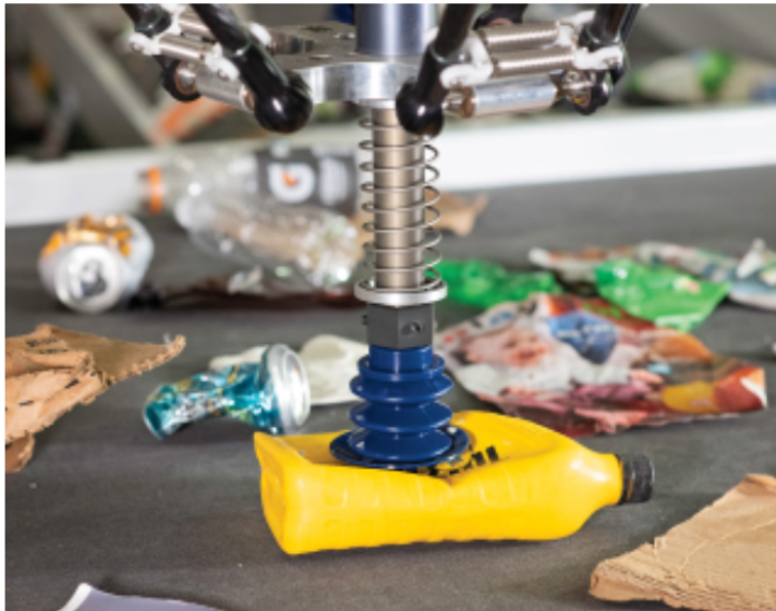
When the belt spots an item, a delta-style arm swoops down and grabs it with a suction gripper. Photo: AMP Robotics
