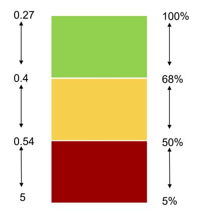
Traffic light for normalized energy index values [kWh/(m3\*100)] and equivalent motor-pump efficiencies [%] for benchmarking (AA13ab - ESAR, Portugal)
