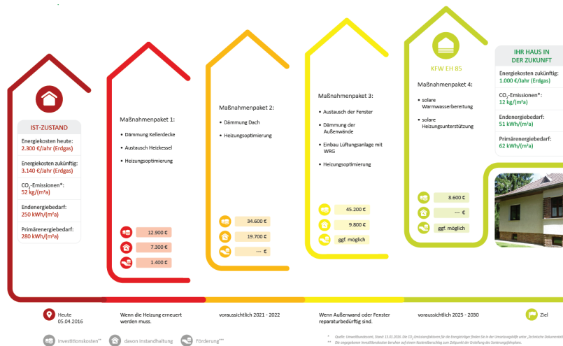
Figure 52: iSPF - renovation roadmap (Source: BMWi)
