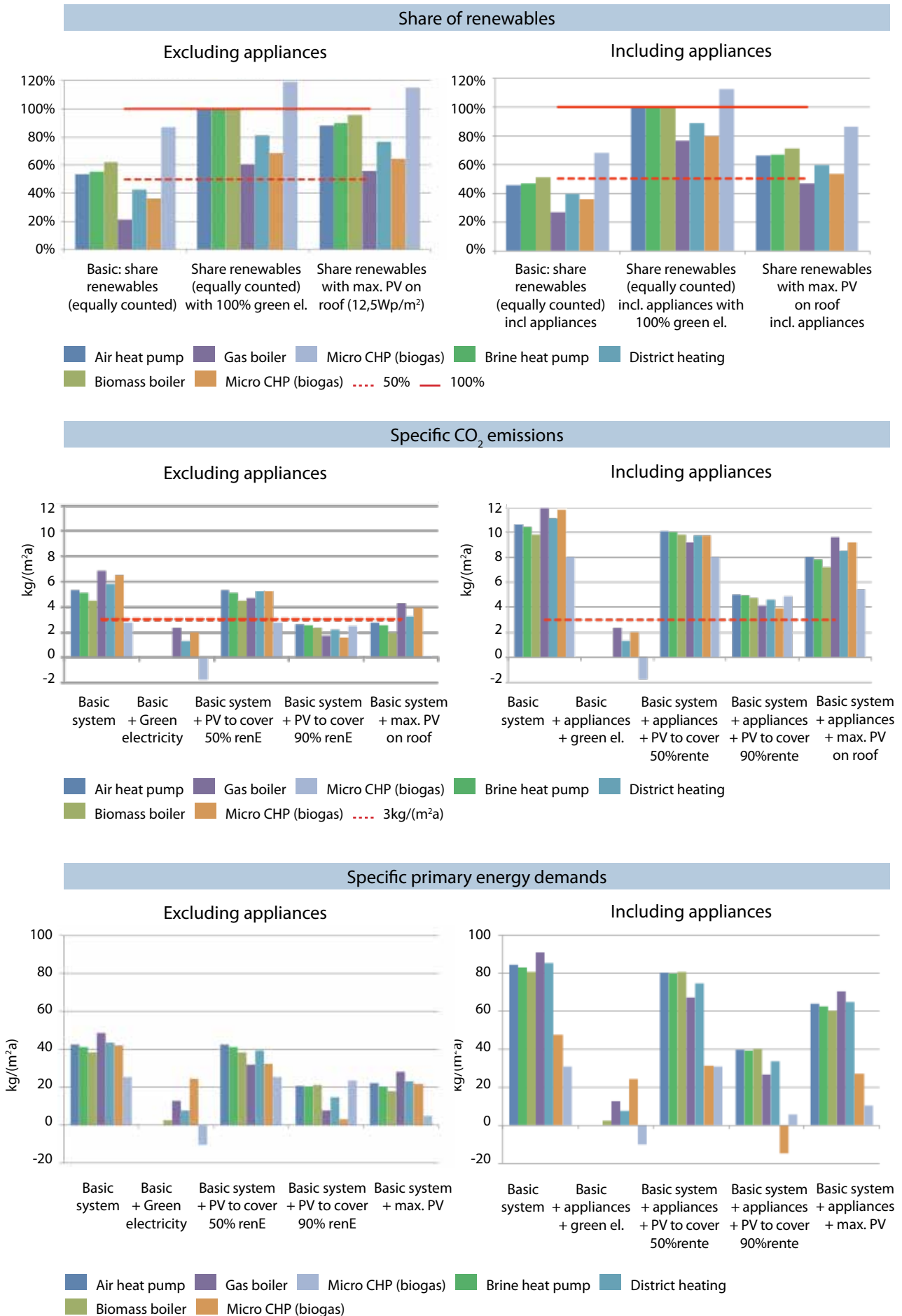
Figure 15: Simulation results for the reference office building in Copenhagen climate zone
