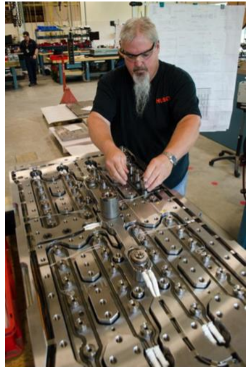
Manifolds manufactured from steel plates. Image courtesy of Husky Injection Molding Systems.
