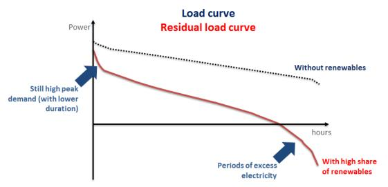
Residual load duration curve for an electricity system with or without high penetration of renewables<sup>1</sup>
