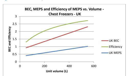
Figure 27 Normalized Efficiency vs. Unit Volume - Chest Freezer - UK BEC
