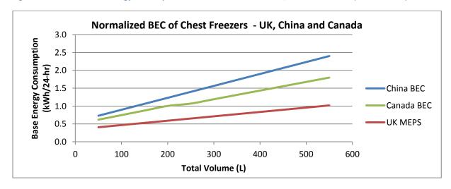
Note that the jog in the Canadian BEC level is caused by a less restrictive requirement for compact chest freezers:
