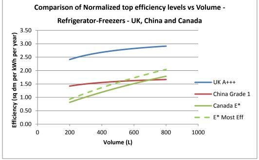
As in the case of Figure 10, the "ENERGY STAR Most Efficient" classification was also included in Figure 15 to give an indication of the improvement in efficiency resulting from a product meeting this new, more stringent requirement (12.5% improvement in efficiency)
