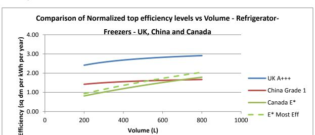
Figure 25 Normalized Efficiencies of small volume and large volume Refrigerator-Freezers at the highest performance level for the UK, China and Canada
