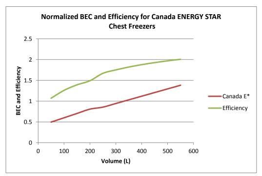
Figure 32 Normalized BEC and Efficiency for Canada ENERGY STAR Chest Freezers
