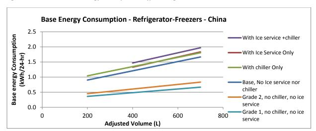
Figure 6 Maximum allowable energy consumption for Type 5 Refrigerator-Freezers 15 - China
