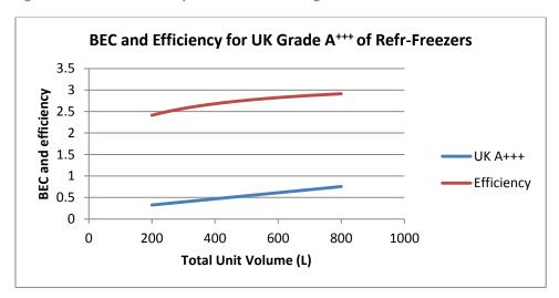
Figure 22 Normalized Efficiency vs Unit Volume – Refrigerator-Freezers – UK Grade A\*\*\*
