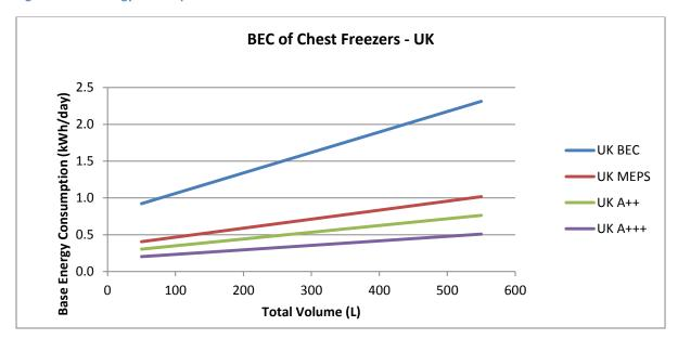
Figure 12 Base Energy Consumption of Freezers for the UK and derived Grade Levels
