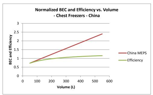
Figure 28 Normalized Efficiency vs Unit Volume - Chest Freezer - China BEC
