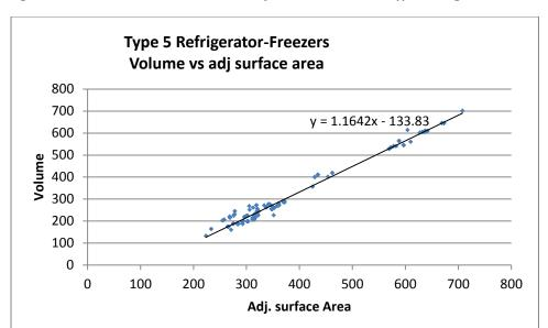
Figure 18 Plot of Total unit Volume vs Total Adjusted Surface Area of Type 5 Refrigerator-Freezers
