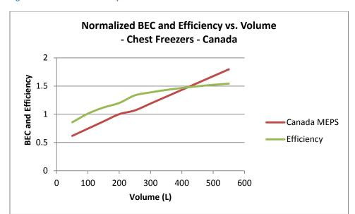
Figure 29 Normalized Efficiency vs Unit Volume - Chest Freezer - Canada BEC
