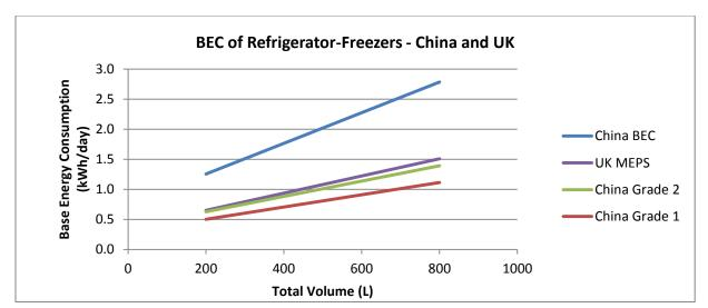
Figure 8 Base Energy Consumption for Refrigerator-Freezers for the UK and China
