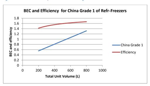
Figure 23 Normalized Efficiency vs Unit Volume – Refrigerator-Freezers – China Grade 1
