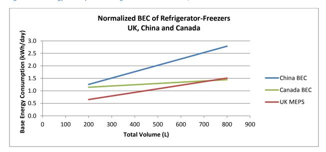
Figure 9 Base Energy Consumption for Refrigerator-Freezers for the UK, China and Canada
