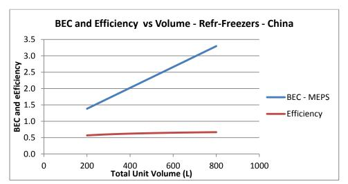
Figure 20 Normalized BEC and Efficiency vs Unit Volume – Refrigerator-Freezers – China BEC (MEPS)
