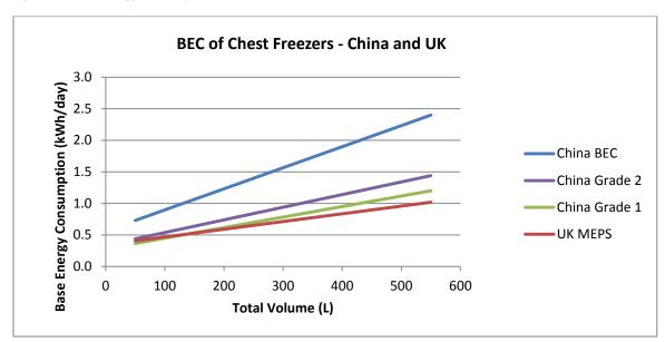
Figure 13 Base Energy Consumption for Chest Freezers for the UK and China
