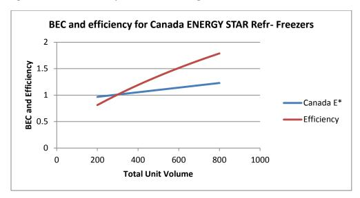
Figure 24 Normalized Efficiency vs Unit Volume - Refrigerator-Freezers - Canada ENERGY STAR
