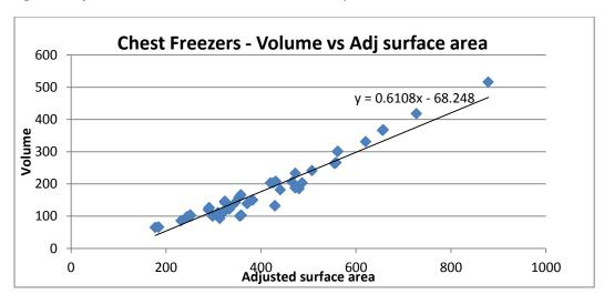
Figure 26 Adjusted surface area vs. Volume for random samples of Chest Freezers from the China Market
