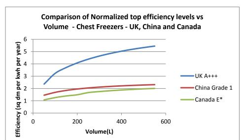
Figure 33 Comparison of Normalized top efficiency levels vs. Volume - UK, China and Canada
