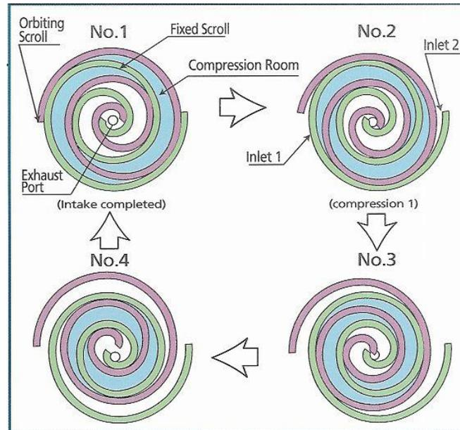
Figure 2-3: Compression cycle in a scroll compressor
