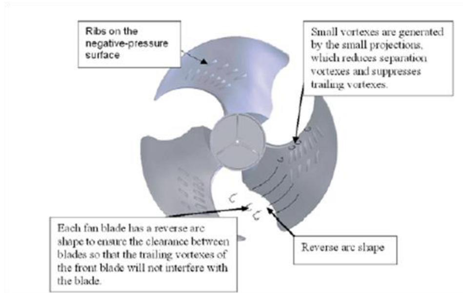
Figure 2-11: Axial Fan Design for A/C Condenser under High Static Pressure
