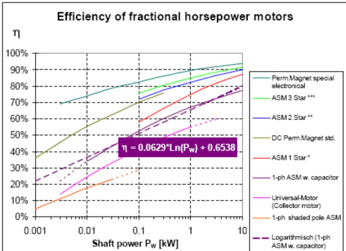
Figure 2-5: Efficiency of fractional horsepower motors
