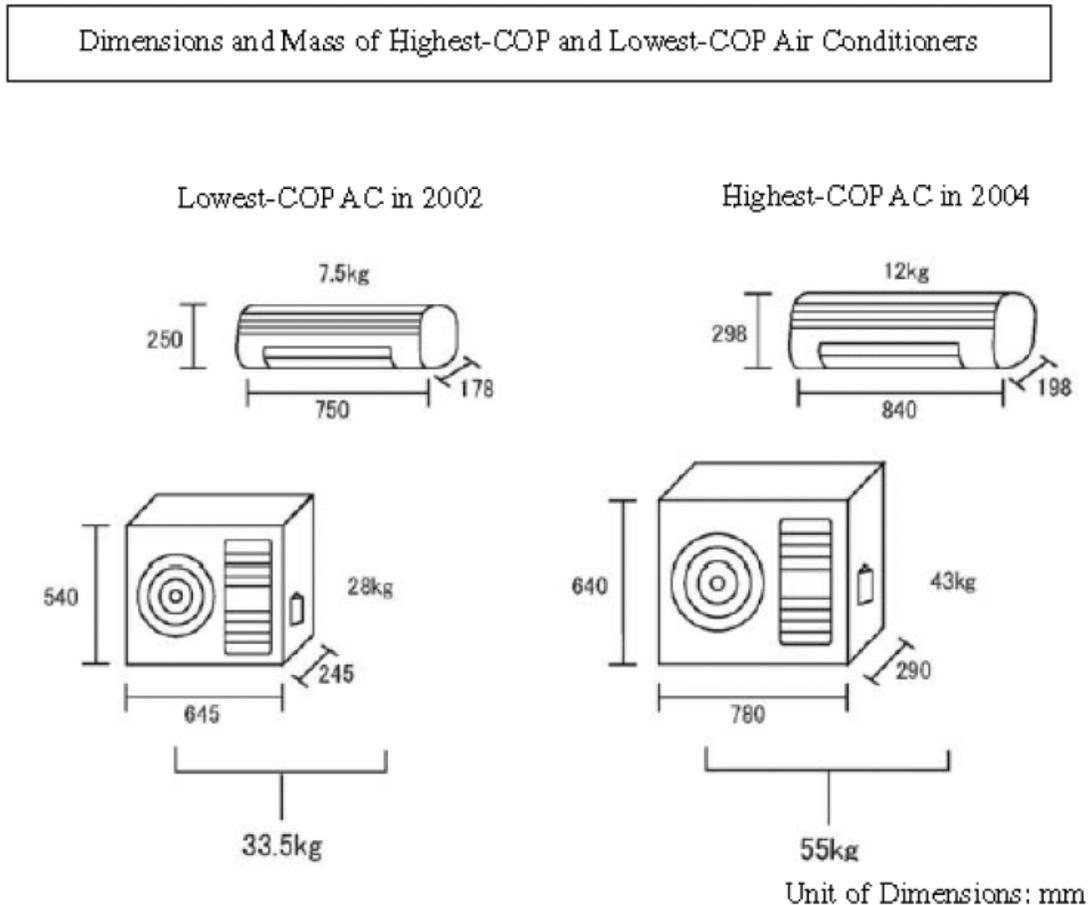
**Figure 2-14: Evolution in mass and dimensions of 2.8 kW AC units in Japan**
