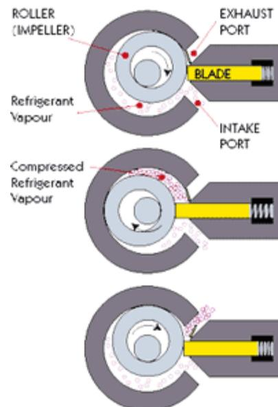
Figure 2-2: Compression cycle in rotary fix-vane compressors
