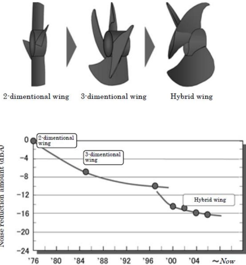
Figure 2-10: Evolution of Axial/Propeller Fan Design
