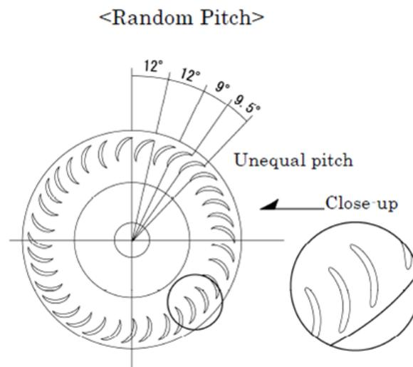
Figure 2-12: Latest Design of Cross Flow Fan Design
