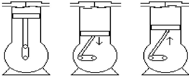
Figure 2-4: Compression cycle in the reciprocating compressor
