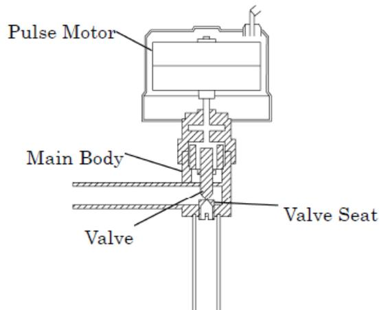
Figure 2-17: Electronic Expansion Valve Schematic
