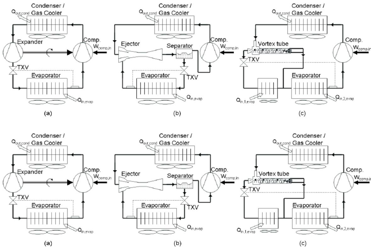
**Figure 2-19: Improvement for low ambient heat pump cycle- (a) Expander cycle, (b) Refrigerant ejector cycle, (c) vortex tube cycle**
