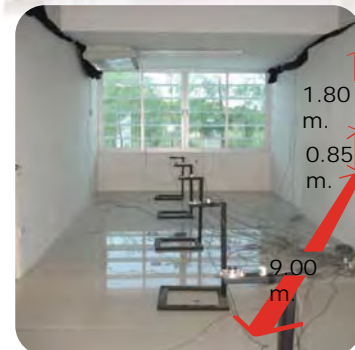
The experimental room with illuminance sensors.
