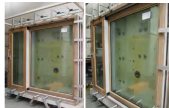
Air Leakage test
