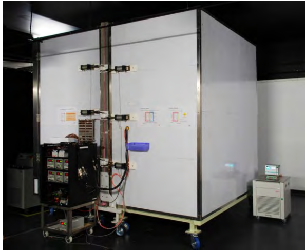
A U-value measurement is in progress
