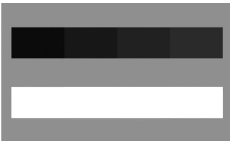
Figure 64: Eight-level grey pattern used in Chinese TV test method
