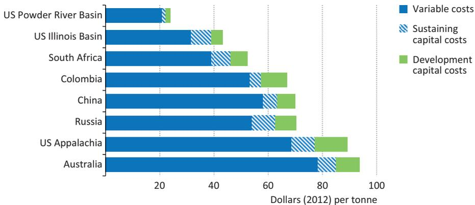
Notes: Based on a sample of more than 400 possible coal mining projects that could become operational by 2024. Cash costs include mining, processing and transport to the main point of sale (not consumption).
