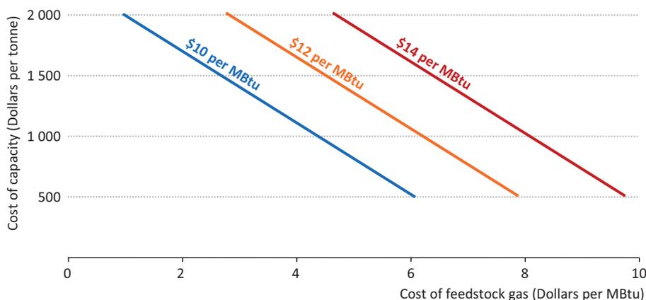
Notes: The calculations here are for a 2-train, 10 million tonnes per year liquefaction facility, operating at 90% capacity, and include costs for a shipping distance of 10 000 kilometres (around \$0.1/MBtu per 1 000 km, depending on the cost of feed gas) as well as regasification (\$0.45/MBtu). The assumed asset life is 30 years and the return on capital is 15%.
