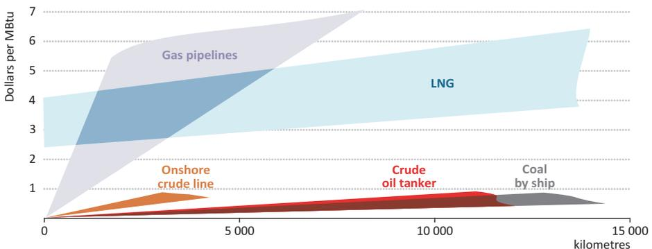
Note: The main determinants of gas transportation costs within the ranges indicated are: for pipelines, the diameter of the pipe and the terrain to be crossed; and for LNG, the initial costs of liquefaction capacity.
