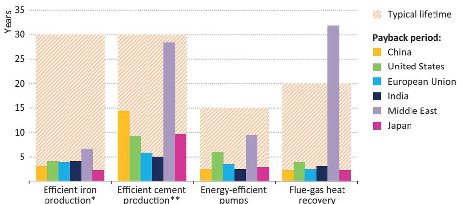
\* Heat recovery from sinter cooler. \*\*Additional pre-heater cyclone stage for a dry kiln.
