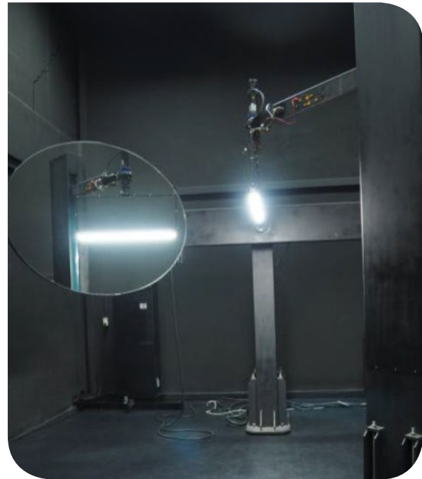
Figure 4 Goniophotometer at Electrical and Electronics Institute laboratory, Thailand (Photograph courtesy of Marie Leroy, UNEP)
