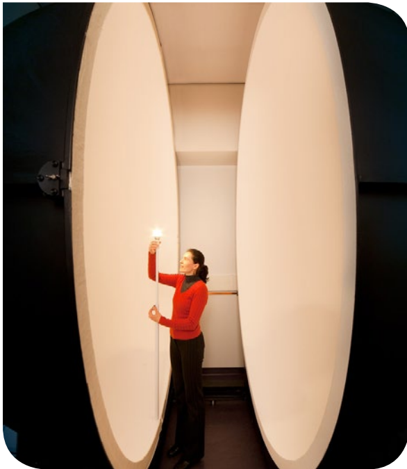
Figure 3 Three metre integrating sphere (Photograph courtesy of VSL, Delft)
