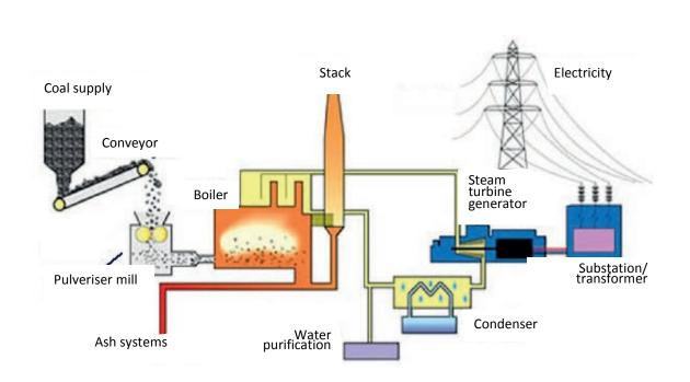
Figure 2 • Schematic of the pulverised coal combustion power generation process
