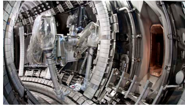
▲ The chamber wall of the Joint European Torus (JET) device was designed to replicate ITER specifications, providing a platform for ITER-relevant experiments.
